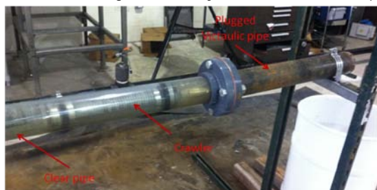
Peristaltic crawler performing an unplugging operation
