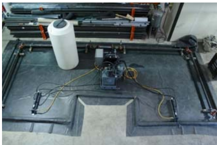
Asynchronous pulsing method: (a) principles of operation (b) bench-scale test bed for asynchronous pulsing
