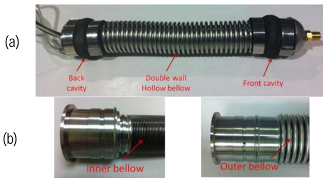
(a) Peristaltic crawler unit, (b) inner bellow assembly (left) and outer bellow assembly (right)
