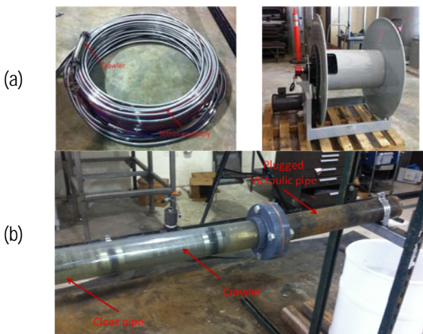
Peristaltic crawler: (a) tether assembly (left) and reel system (right), (b) Peristaltic crawler performing an unplugging operation
