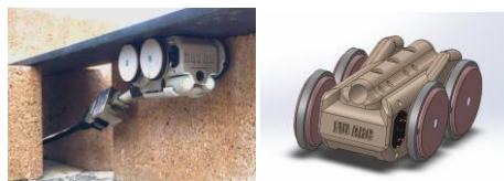
Pneumatic pipe crawler.
