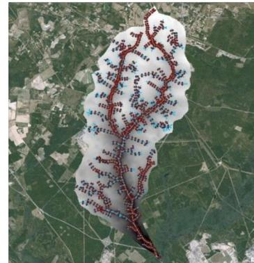
**Fig 2. Cross sections of streams and tributaries in Tims Branch watershed that are directly exported from ArcGIS into MIKE 11**
