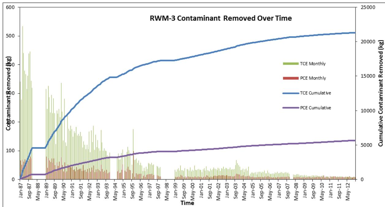
**Fig. 2. Recovery of TCE and PCE from 1987 to 2012 from Recovery Well #3 as indicator for the need to optimize pumping from every well.**
