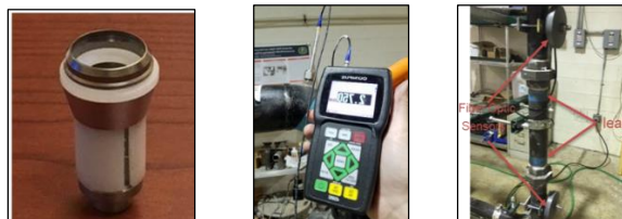
Erosion Coupon, Thickness measurement, Fiber-optic Sensors
