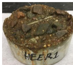
Aged concrete with exposed rebar and aggregate protrusion-weight loss graph with and without erosion effect
