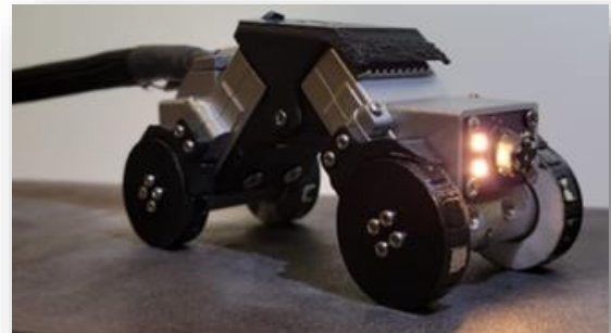
FIU’s Mini-Rover Inspection Tool
