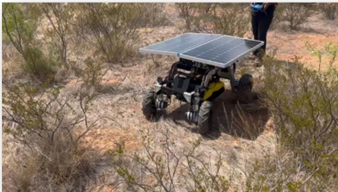
Large Area Robotic Inspection Tool with GPR technology – Inspection of LM sites
