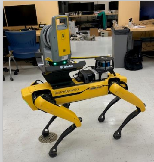
Digital Decommissioning Boston Dynamics SPOT and Trimble X7 technologies
